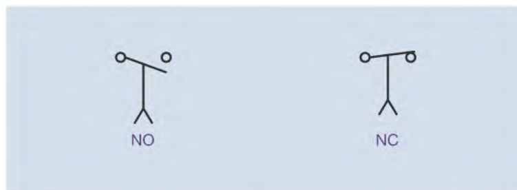
Figure 11–1 On-delay normally open and normally closed contacts.
