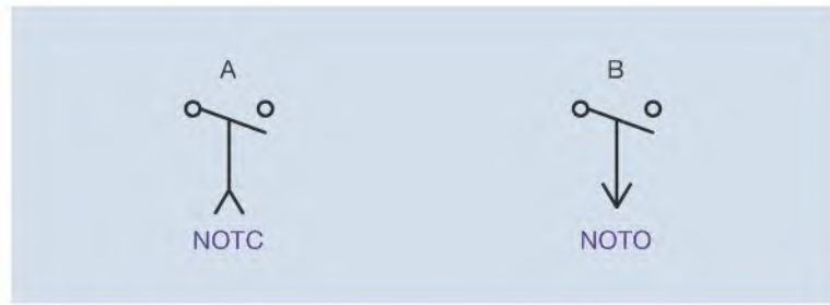
Figure 11-5 Contact A is an on-delay contact with the abbreviation NOTC (normally open time closing). Contact B is an off-delay contact with the abbreviation NOTO (normally open time opening).
