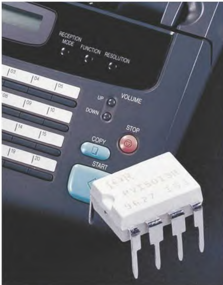
Figure 5-22 An 8 pin integrated circuit containing two low power solid-state relays.
