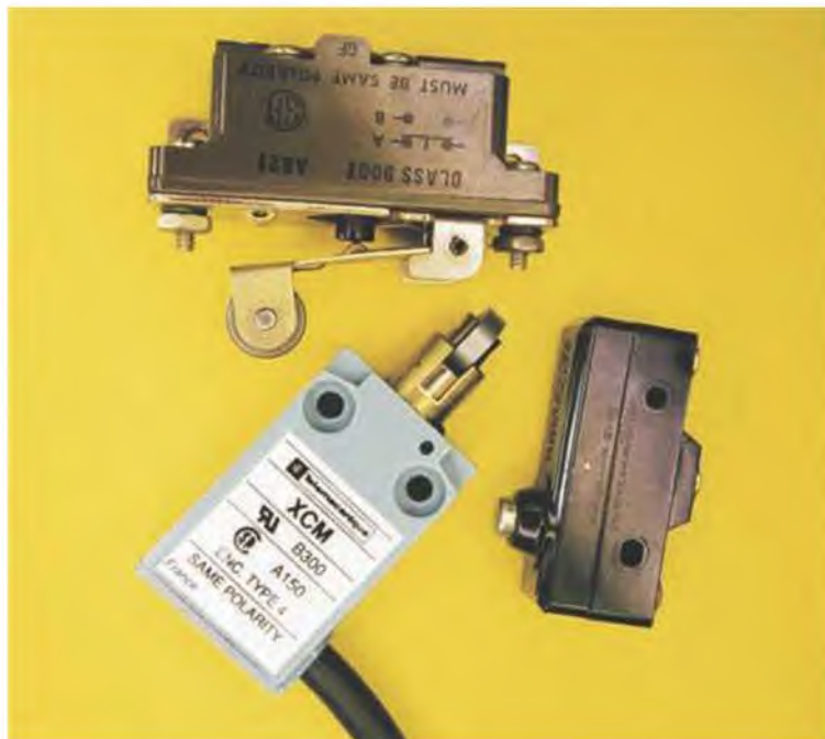
Figure 16-7 Micro switches can be obtained with different types of activating arms.
