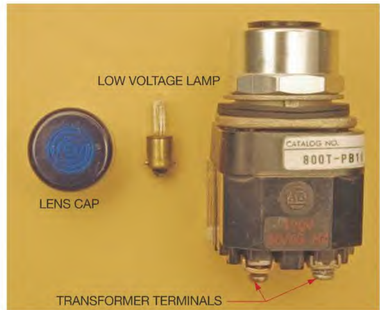
Figure 2-18 Illuminated push buttons generally employ a small transformer to reduce the control voltage to a lower value.
