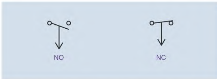
Figure 11-2 Off-delay normally open and normally closed contacts.
