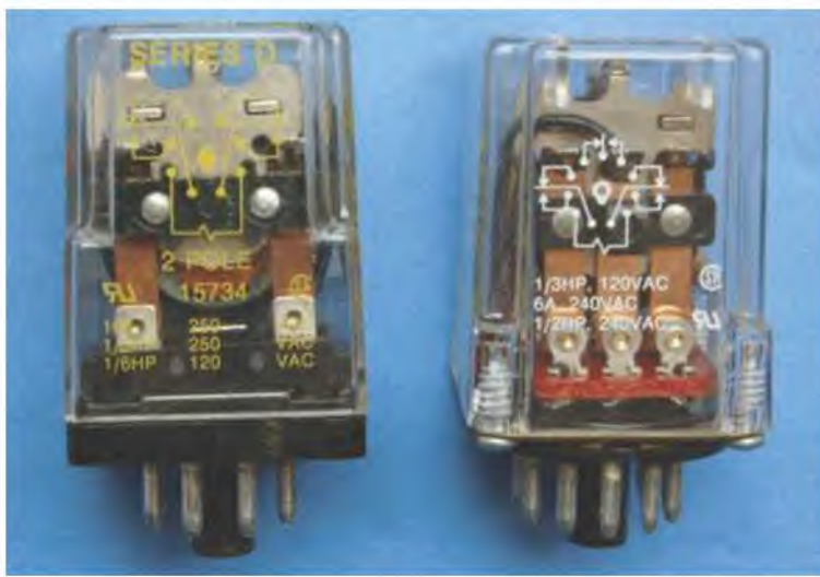
Figure 5-16 Relays designed to plug into 8 and 11 pin tube sockets.
