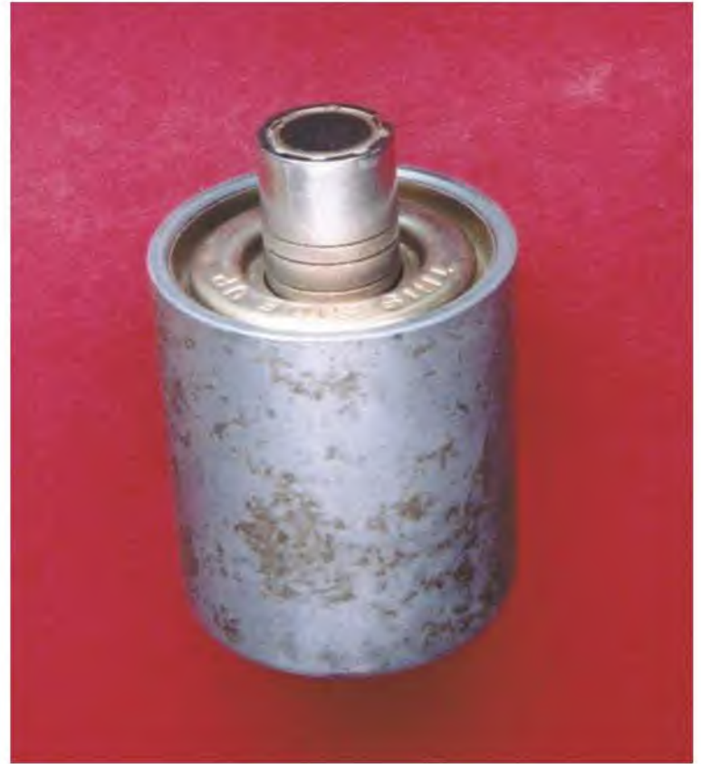
Figure 4-27 The line on the shaft that represents the desired amount of current is set flush with the top of the dashpot container.
