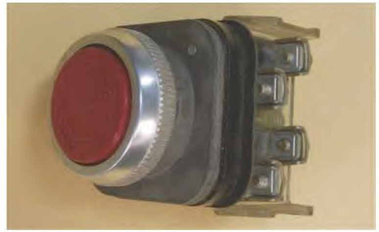
Figure 2-7 Double acting push buttons have four terminal screws.
