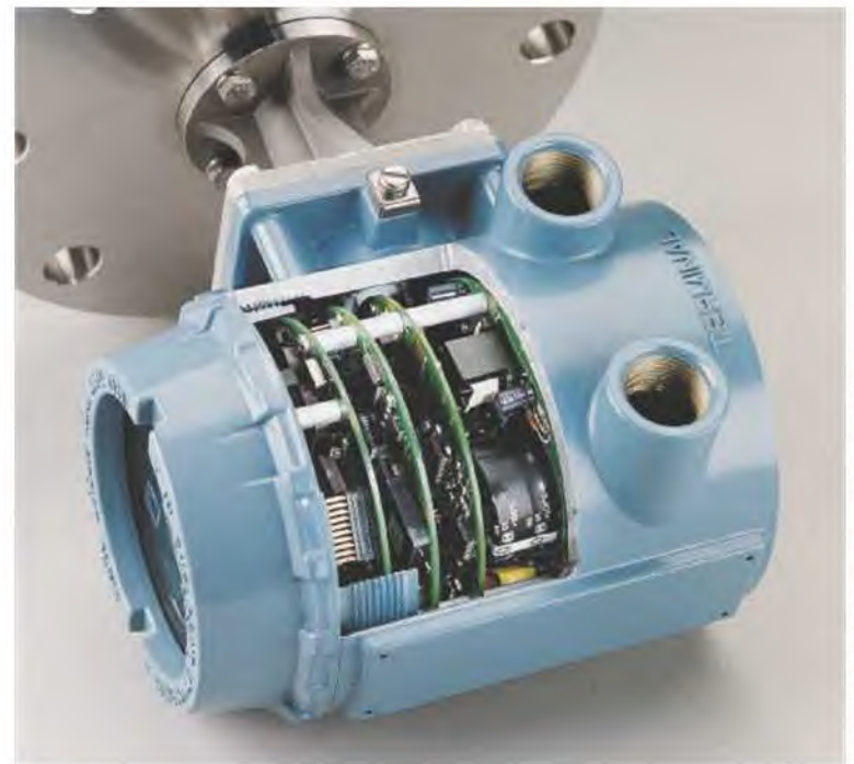
Figure 14-8 Cut-away view of a microwave level gauge.
