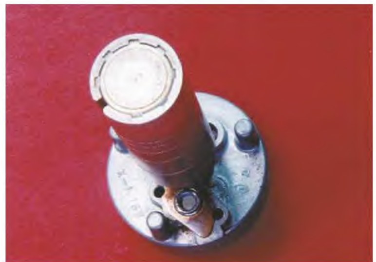
Figure 4-22 Setting the opening of the orifices affects the time delay of the dashpot timer.
