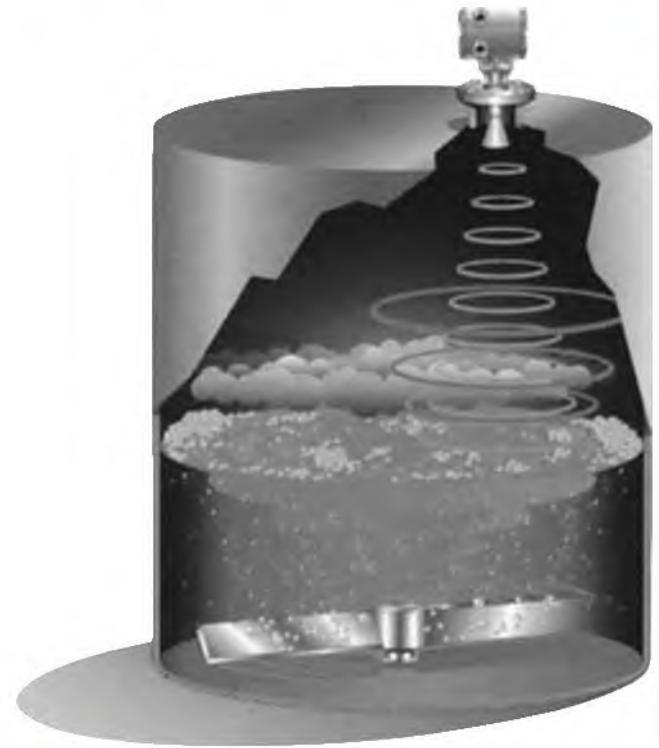
Figure 14-7 Operation of the radar gauge.
